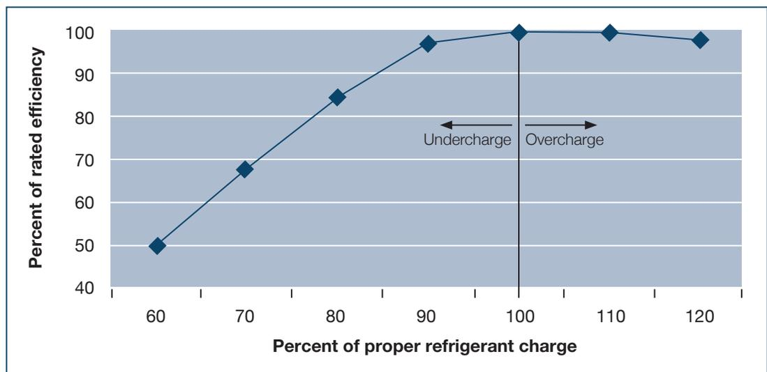
**Figure 1. The effect of refrigerant charge on efficiency.<sup>1</sup>**
